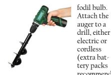
recommended). You can quickly make a hole of the required depth, drop in a bulb, backfill with soil, and repeat.
